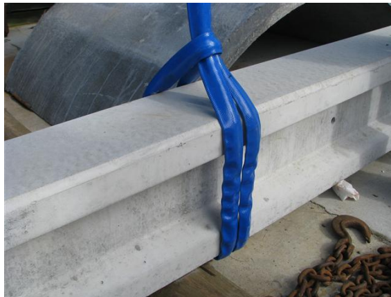
Using a choked polyester or composite material sling
